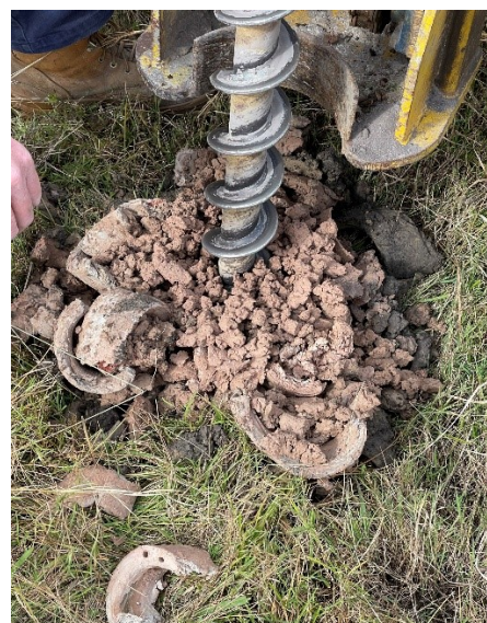
The cuttings from BH5 encountered topsoil, overlying alluvial and residual soils
